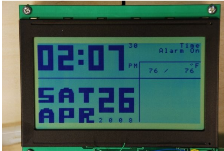
Figure 27: Main Screen with Alarm On and Fahrenheit Temp
